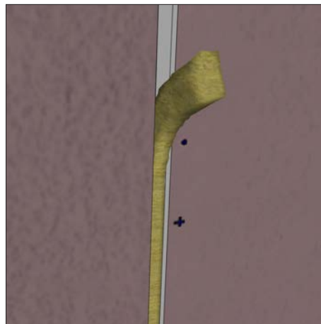
3/4" Gap or Greater, or Expansion Joint
